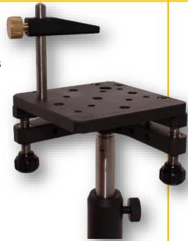
The KPMSS100 and KPMS100 included a prism platform and a clamping arm as a prism mounting hardware. This mount is designed to integrate many prisms, cube beam splitters and corner cubes into any optical system. This model mount can be used for aligning components that require tilt adjustment.
